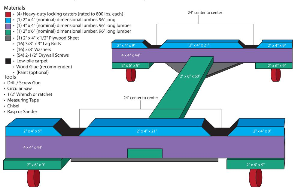
Note: These plan are provided as general guidelines to help you build a chassis dolly to support the building of a Factory Five Racing Mark IV Roadster.
